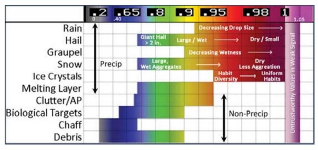
**Fig. 2**. Typical CC values for common targets sampled by dual-polarization meteorological radars. Taken from NWS WDTD Radar and Applications Course CC training material.
